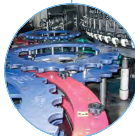
Filler and capper conveyor system
